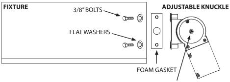
TORQUE TO 25 FT LB (DO NOT EXCEED); THIS SHOULD NOT BE EXCEEDED AS IT COULD CAUSE DAMAGE. THIS PRODUCT WAS DESIGNED TO MOUNT TECHLIGHT PRODUCT WEIGHING UP TO 65 POUNDS. ANY ATTEMPT TO EXCEED THIS WEIGHT AMOUNT MAY CAUSE FAILURE.
