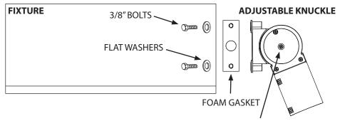
TORQUE TO 25 FT LB (DO NOT EXCEED); THIS SHOULD NOT BE EXCEEDED AS IT COULD CAUSE DAMAGE.
