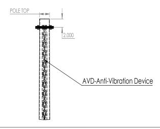
**For Refrence Only:** The ASCE 7 Hazard Tool is the official source of information for pole selection when identifying wind speed zone limits within North America.
