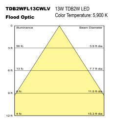
\*Delivered lumens shown do not include light loss due to the fixture grill or lens.
