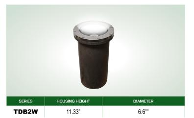
**MOUNTING** — Fixtures are designed to be in-ground burial lights and should be installed according to the installation instructions made available by Techlight. Proper drainage and substrate must be provided for water to flow freely through the well sleeve. A  $\frac{3}{4}$  conduit entry is supplied into the anti-siphon chamber of the housing. Conrete pour kits available (see Accessories).
