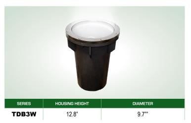
MOUNTING - Fixtures are designed to be in-ground burial lights and should be installed according to the installation instructions made available by Techlight. Proper drainage and substrate must be provided for water to flow freely through the well sleeve. A 3/4" conduit entry is supplied into the anti-siphon chamber of the housing. Conrete pour kits available (see Accessories).
