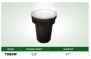
**MOUNTING** — Fixtures are designed to be in-ground burial lights and should be installed according to the installation instructions made available by Techlight. Proper drainage and substrate must be provided for water to flow freely through the well sleeve. A ¾" conduit entry is supplied into the anti-siphon chamber of the housing. Conrete pour kits available (see Accessories).
