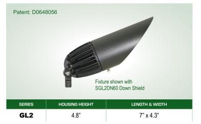
**MOUNTING** — The die cast aluminum mount is secured to the heat sink by stainless steel screws and is sealed with an integral o-ring, A ½" threaded knuckle is provided standard.
