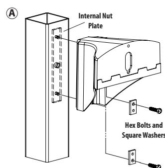
Pull the fixture whip into the wiring chamber of the mounting arm and align the bolt retaining hole
